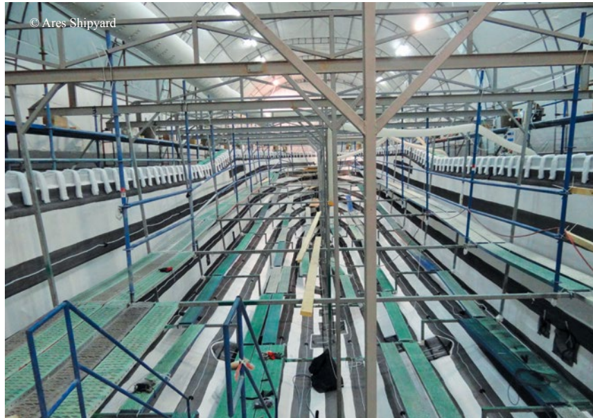
35m composite hull ready for infusion
